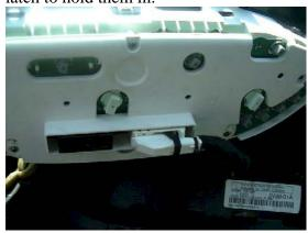
(after unplugging the cables, the whole cluster comes out, which you can work on away from the car... on a desk or such.)
