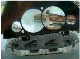
The Gauges are designed to be installed over the needles without having to remove them This has a few benefits, one being not having to calibrate your needles(could become a headache)
