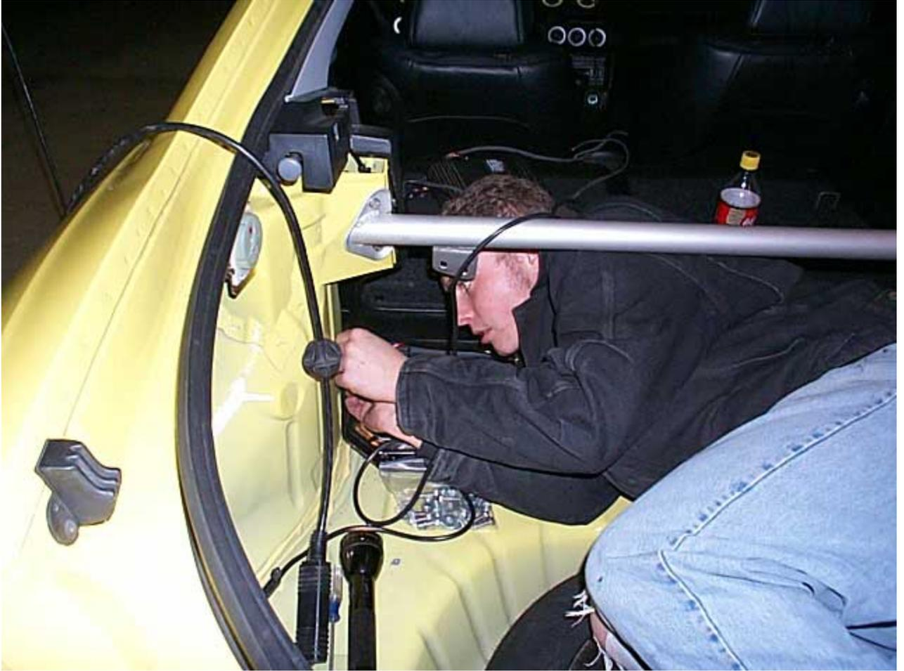
11. When done doing both "L" backing plates, drill out all the other holes for the lower brackets. Do not drill down to far on the right side, there is some lines there, they are protected, but just don't sit there and play with the drill through the hole.
