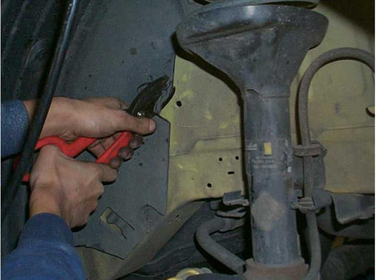
10. Now remove the cross bars from the lower brackets, line up the brackets, and have the other person line up the "L" backing plate. This backing plate will cover the holes in the actual strut tower for the bracket. You line it up from inside the wheel well. Put the bolts in, you may notice a little difficulty doing this, at least we did, what we did to solve it, is use the slightly larger drill bit and bore out the holes just a little more that we made on the body panels.
