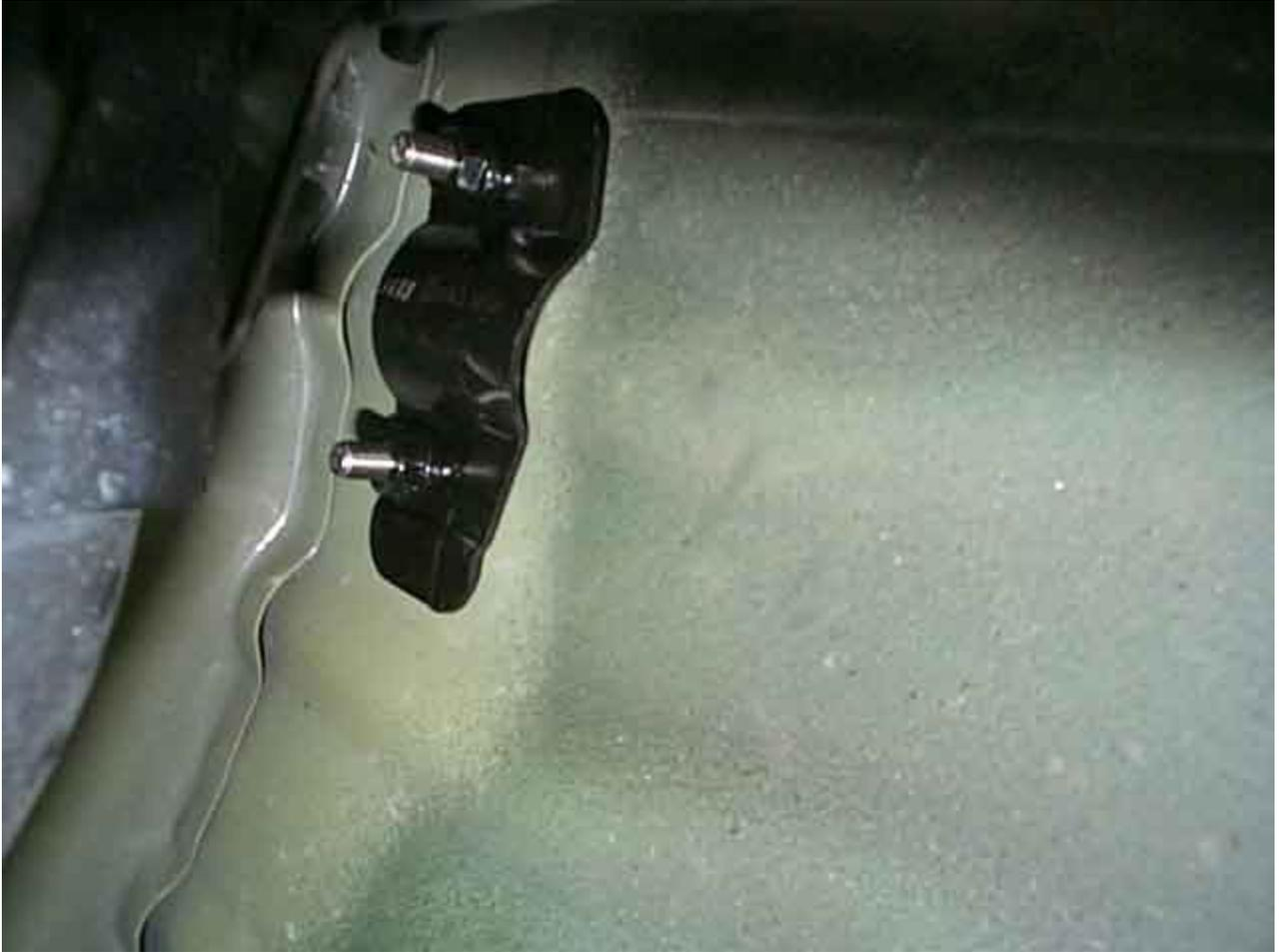
13. Now do the mid-size backing plate. This backing plate covers the front holes of the bracket. To get to this one you may need some small hands and a little fiddling to line it up right but it's very possible. Do to this one you may also need to just remove the main bushing brackets for the rear sway bar to get your hands in. On the Left side it's almost a must. The main bushing brackets are 15mm I think, and there are just one per side.
