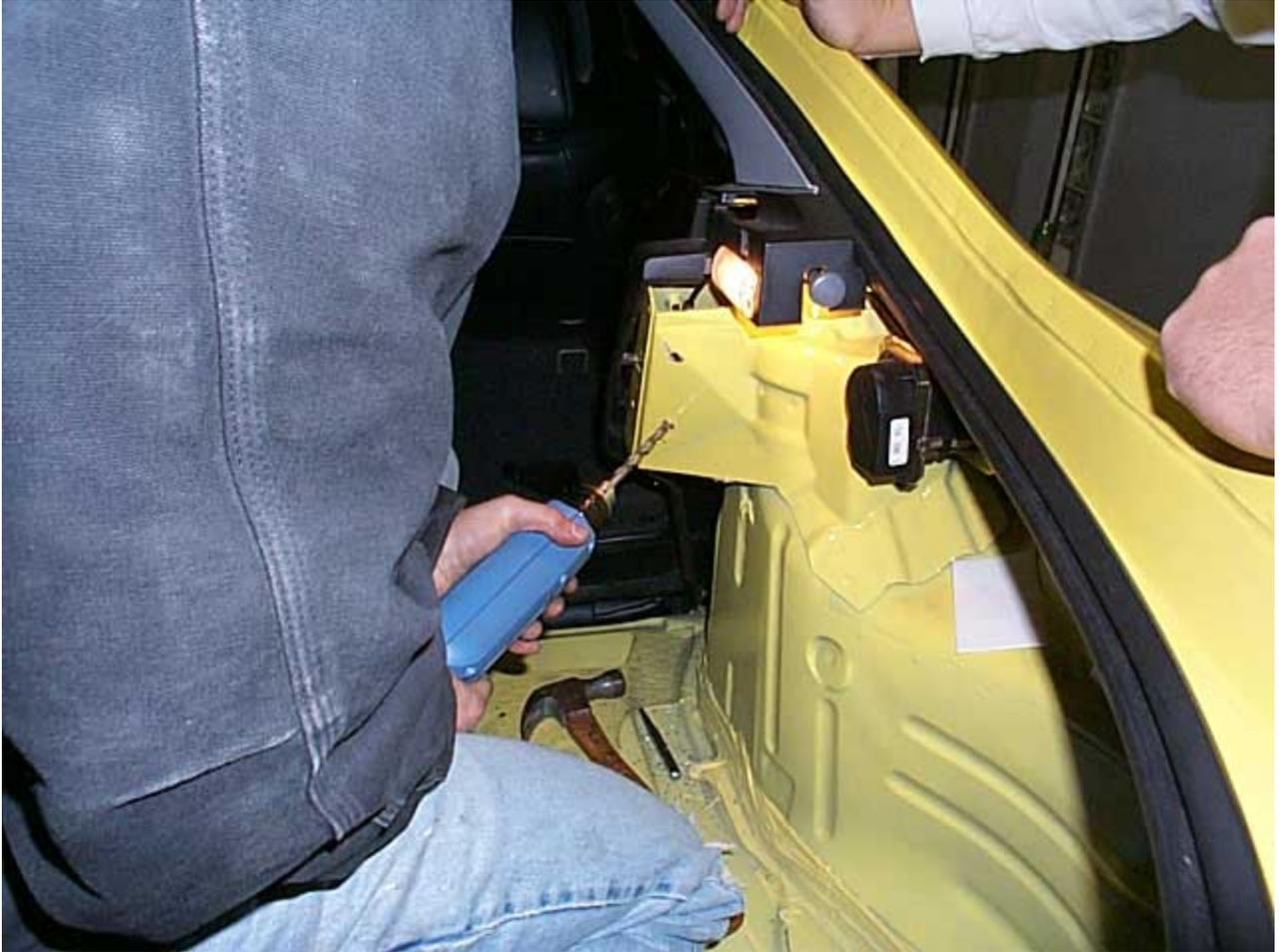
6. Put bar back, hold the triangle backing plates from the bottom and put the bolts in loosely. Don't worry when you are done you tighten everything down.
