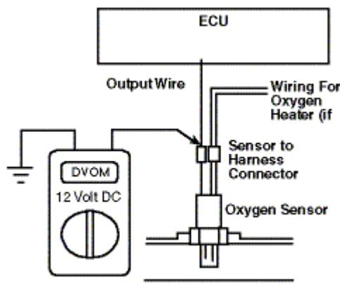
Even though you can't see the number of cross-counts without a scanner, you can use a digital voltmeter to watch the open/closed loop system operate. Just connect your meter as Illustrated above, while the O2 sensor is still connected, and start-up the car.
