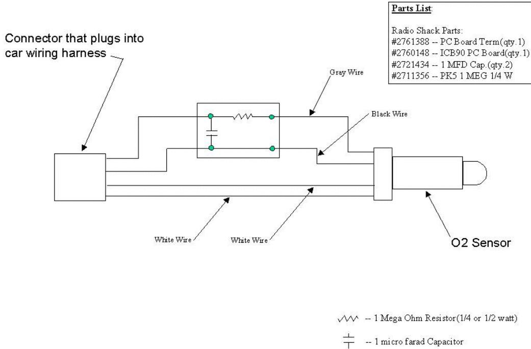
Assemble the components on the project board and trim it to fit, then connect the wires from the o2 sensor to the correct inputs on the circuit. Reinstall your o2 sensors and reset the computer (disconnect the battery for 5 - 10 minutes) and you should be MIL light free.
