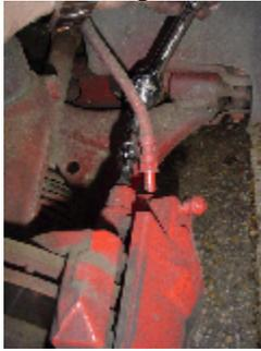
4. After you remove both sockets rest the caliper on top of something to keep the flexible brake line from being pulled off and then needing to bleed the brakes if this were to occur.
