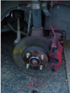
2. Remove cap both caps to detach the main part of the rotor. You will need a 7mm Hex Socket to remove these. This can be found at AutoZone for \$3-\$4.
