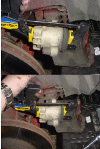
7. After you have finished compressing the plunger set the caliper back down on the rest and unscrew the retaining clips that you sprayed a little bit ago. You can either unscrew them or break them off. To unscrew them use a flat head and place it in the bent pieces of the clips and tap on it lightly with a hammer to get it started. You can unscrew it the rest of the way by hand.
