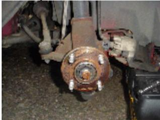
9. Place on your new rotor and if you unscrewed the retaining clips, screw them back on.
